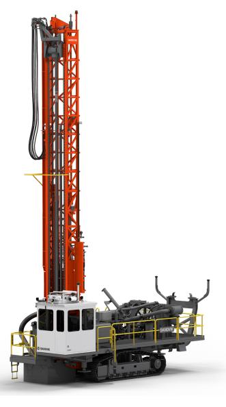
Sandvik D50KX is a diesel-powered, self-propelled, crawler-mounted blasthole drill for surface mining. it is standard equipped for rotary with optional down-the-hole (DTH) hammer drilling power.
