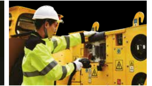
Type (combo) 1 or 2 for Combined Charging System (CCS) connectors. Charging anywhere in the mine both on-board and off-board.
