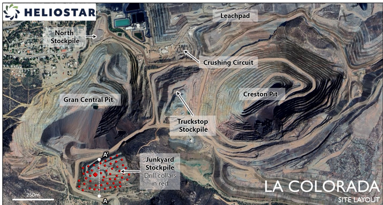
Figure 1: Plan Map of the La Colorada Mine with pits and stockpiles/waste dumps, Junkyard drill collars, crusher circuit and leach pad location shown.
