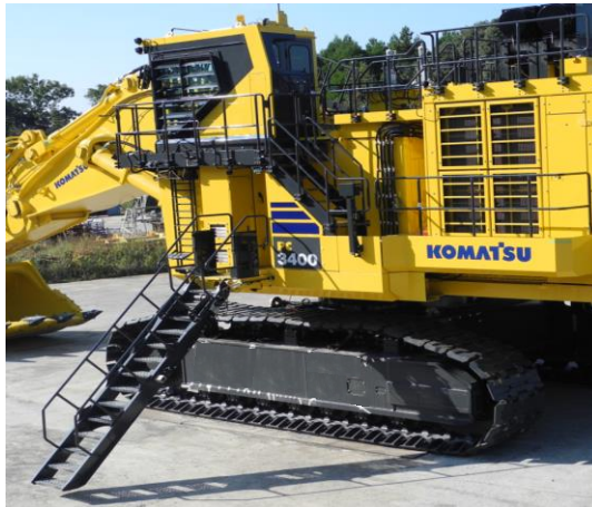
Main access ladder
