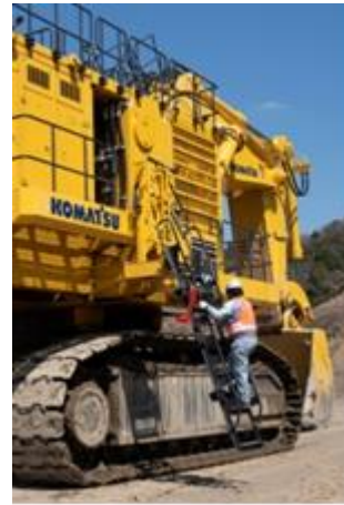
Emergency escape ladder
