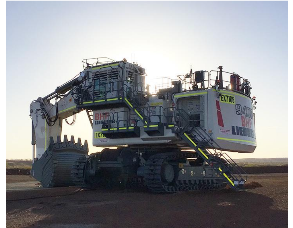
9400E electric excavator on site at Yandi mine in February 2024
